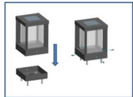
Step 3 : Place the lantern on the base and lock it by 4 supplied screws.
