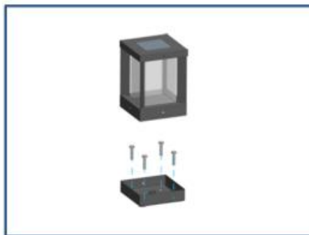
Step 2: Remove the base from the lantern and Mounted the base onto the deck / ground with screws (supplied).
